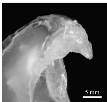
Figure 3. Translucent residue of chitin following extended immersion of Dosidicus beak in alkaline peroxide.
